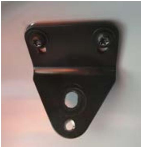
2.7) To the inside roof of the canopy in four locations, **use hardware in the base rack or roof bar fitting kit** to assemble the two M8 x 35mm Torx bolts (6151881) with two flat washers M8 x 19 through the top internal frame brackets (37500309) by pushing the bolts through the holes in the bracket and foam pad seals through the spacers in the roof of the canopy and **secure as per the base rack or roof bar installation instructions.**
