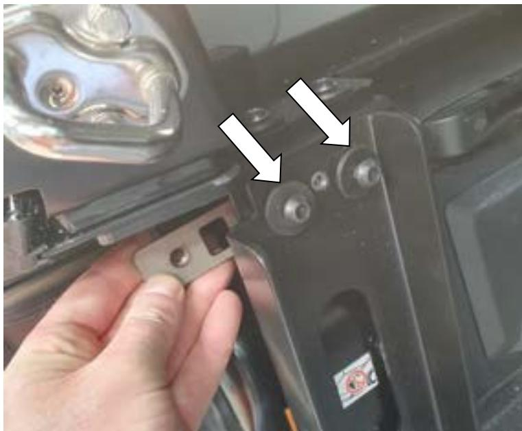
1.2) Assemble the left-hand rear tub support bracket (667PD022L) in the left-hand rear corner of the tub. Align the top end of the bracket with the existing slotted holes in the canopy's rear mounting bracket.
