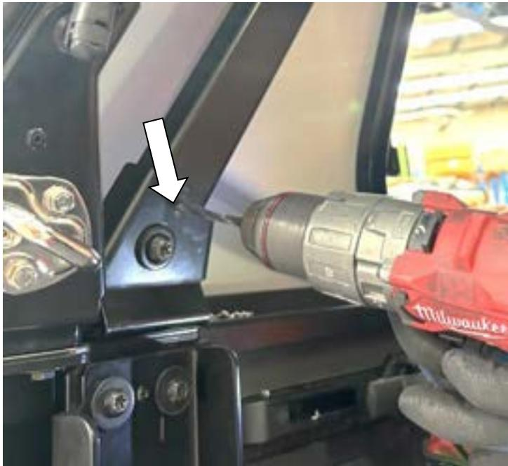
2.13) At both the top and bottom internal frame brackets drill 5.2mm holes through the existing holes in the upper and lower internal frame brackets through the stay brackets. (Eight places total).
