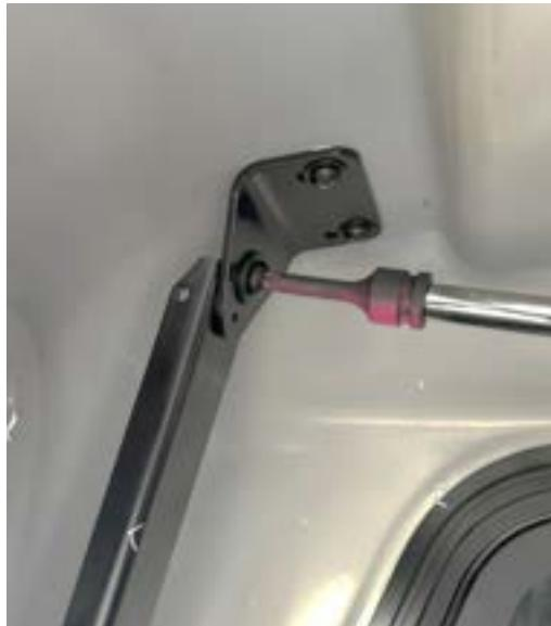
2.8) At the front left-hand side inner roof area of the canopy, locate the shorter length front stay internal frame bracket (667AQ008) behind the top internal frame bracket. Install an M10 x 30 Trox screw (6152149) with an M10 x 25mm flat washer (4584399) through the hole in the top internal frame bracket into the weld nut on the front stay internal frame bracket. **Loosely tighten.**
