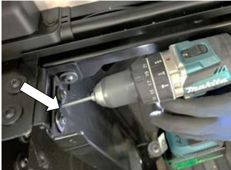
1.20) Install pop rivets (6609101) into the drilled holes on each side of the tub.
