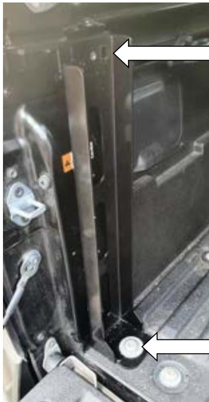
Locate the top holes of the bracket to the existing rear canopy mounting bracket.
