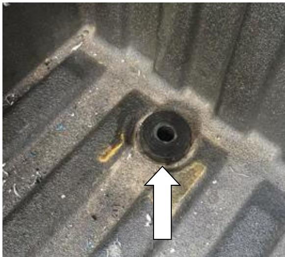
1.10) At the front corners of the tub (where the M12 bolts were previously removed), place the round 46 OD x 12mm thick spacers (6253453) over the holes.
