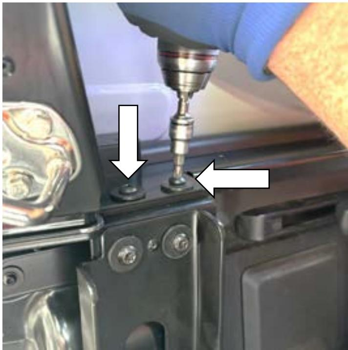
2.3) At the rear of the left-hand base rail inside the canopy, remove the M8 Torx bolts on top of the base rail. Discard the bolts **but retain the washers and M8 nut plate.**
