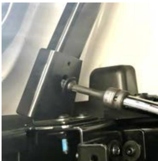
2.9) Position the bottom end of the front stay bracket (667AQ008) behind the lower left-hand internal frame bracket (6582549L). Install an M10 x 30 Trox screw (6152149) with an M10 x 25mm flat washer (4584399) through the hole in the lower internal frame bracket into the weld nut on the front stay internal frame bracket. **Loosely tighten.**
